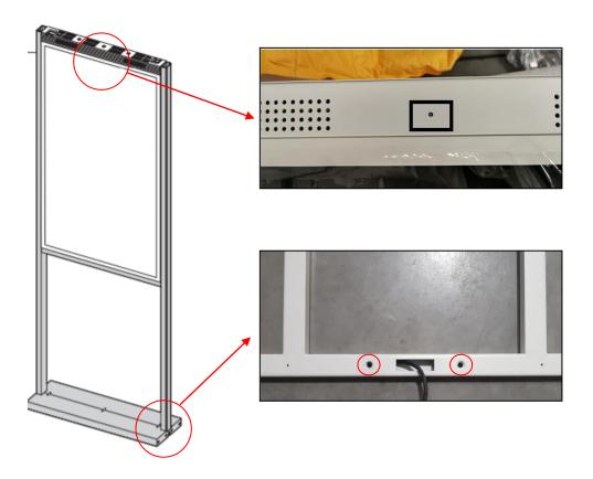
**Step 7**Place the covers on the base after attaching the screen and screw them together on both sides.
