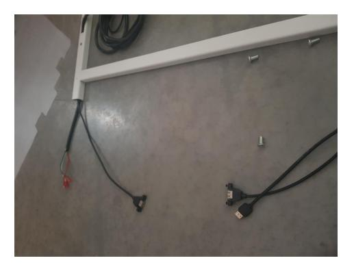
Feed the USB and HDMI cable into right side. You can also feed a LAN cable through if needed.
