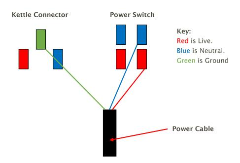
Make sure the connections match with each respective type. I.e. Live cables connect to Live connection points. Please do not remove the plastic covering on the end of the cables.
