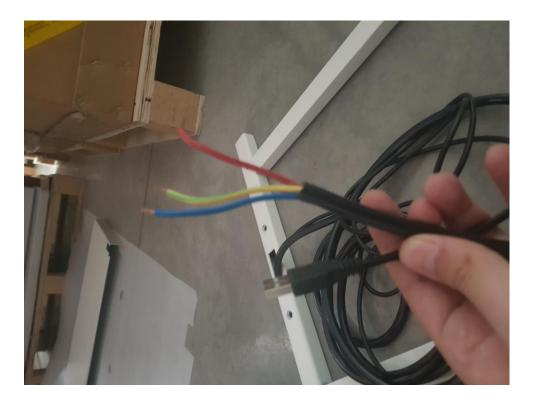
**Step 3**Connect the cables fed through the bottom of the base to the base cover that has the switch attached to it. When connecting the power cable, please make sure it looks exactly like below.
